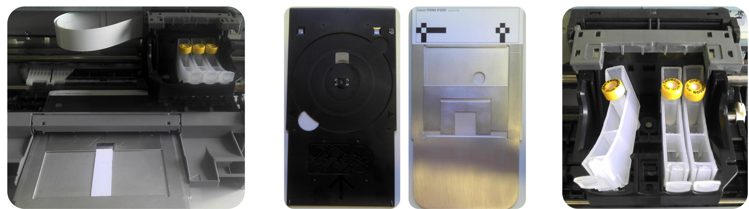
Fig. 2 Modified printer with the original tray guide, removed paper feed assembly, dismantled sensors and transport slide cut out allowing the contactless movement of all plate formats (left); original CD-tray and custom-built plate tray (center); print head carrier with Thomson SINGLE StEP® Filter Vials as sample reservoir in cartridge adapters (right)
