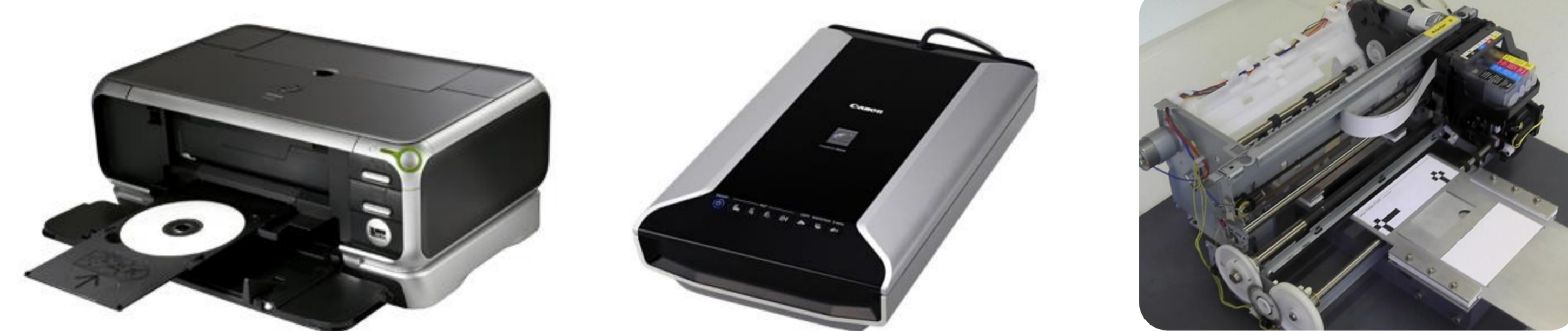
Fig. 1 Canon Pixma 3000 with original CD-tray, Canon CanoScan 9000F and modified Pixma 3000 and custom-built plate tray with mounted 10 x 5 cm thin-layer plate in the new tray guide system
